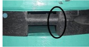
Sloping side not visible OK
